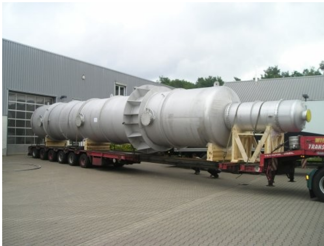
Vacuum Distillation Coloumn
